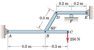
4/83 Determine the magnitude of the pin reaction at A and the magnitude direction of the force reaction at the rollers. The pulleys at C and D are small.
